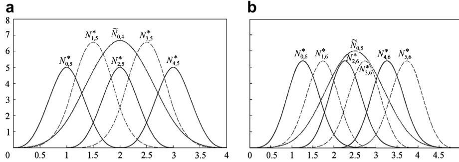
Fig. 1. The images of B-spline basis functions defined over  $T$  and  $T^*$ . Dot lines denote  $\tilde{N}_{0,k}$  defined over  $T$ , solid lines and dash lines denote e-kind and o-kind of  $N_{i,k+1}^*$  defined over  $T^*$ , respectively. (a)  $k = 4$ ; (b)  $k = 5$ .
